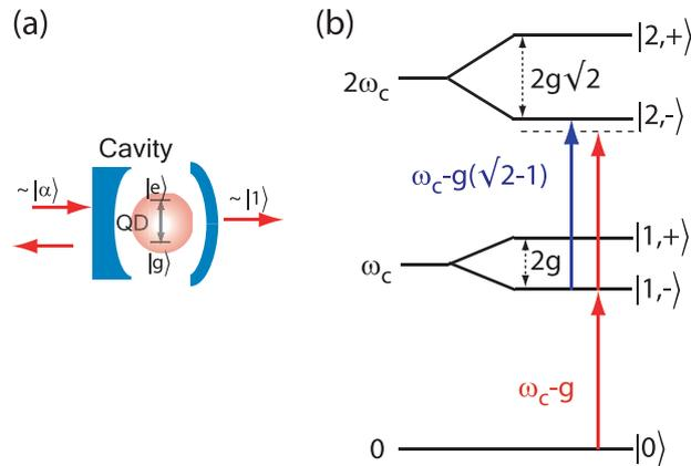
**Figure 2.** (a) Schematic representation of an optical cavity strongly coupled to a single quantum emitter. In photon blockade operation, a coherent state is incident on one side of the cavity and single-photon states exit at the other side. (b) Diagram showing the anharmonic ladder of energy eigenstates of a strongly coupled system.
