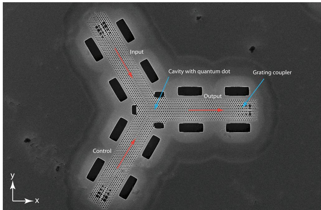
**Figure 9.** The photonic crystal network integrating three waveguides coupled to a single photonic crystal cavity. This device could be used for all-optical switching where the signal and control beams come from different ports on the chip.
