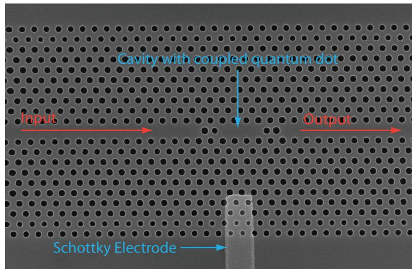
**Figure 6.** Integrated electro-optic switch (concept device) for on-chip optical signal processing. The transmission function is controlled using a single QD coupled to the cavity. The QD frequency can be changed using a bias electric field applied via a Schottky electrode.
