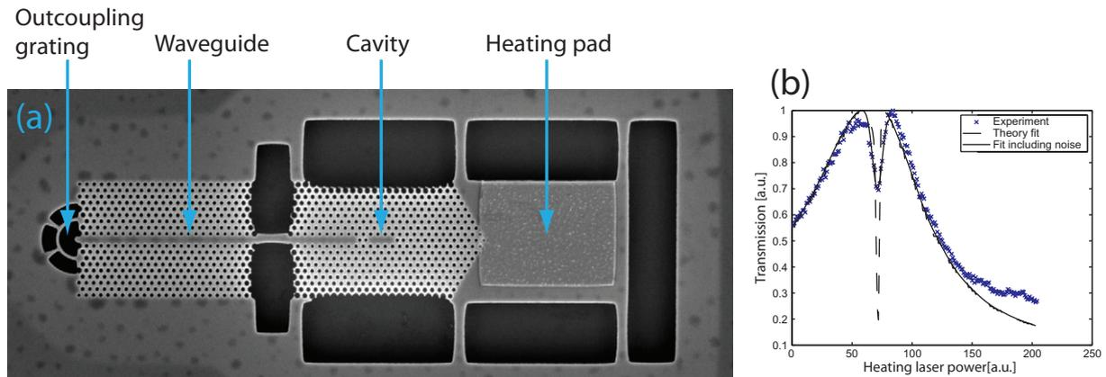
**Figure 5.** (a) The photonic crystal device integrating a cavity coupled to a waveguide that is terminated with a grating for efficient light scattering. An external laser beam focused directly on the metal heating pad on the left is used to locally control the temperature of the device that is correlated with the cavity and QD wavelength. (b) Transmission measurement showing the Lorentzian spectrum and the drop in transmission caused by the coherent interaction with the QD.
