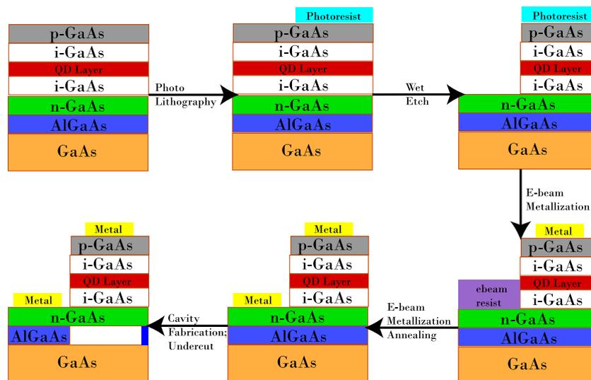
**Figure 7.** Fabrication steps for contacts and photonic crystal devices enabling electrical control in a p–i–n junction. Here, p-GaAs, n-GaAs and i-GaAs indicate p-doped, n-doped and intrinsic gallium arsenide, respectively.
