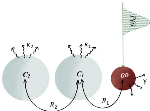
**Figure 2.** System schematic for population dynamics. The colloidal QD which has a radiative decay rate  $\gamma$  is pumped with an incoherent pulse  $P(t)$ . The population transfer between the colloidal QD and  $C_1$  occurs with a rate  $R_1$ .  $C_1$  has a decay rate of  $\kappa_1$ . Population transfer rate between  $C_1$  and  $C_2$  is  $R_2$ .  $C_2$  decays with a rate  $\kappa_2$ .
