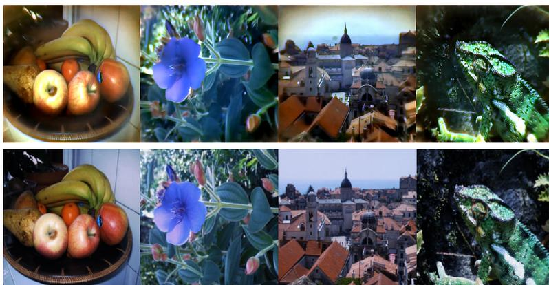
Top: Design framework to co-optimize a meta-optic and reconstruction algorithm via a differentiable pipeline. Middle: Images captured using a single 500- $\mu\text{m}$   $f/2$  meta-optic. Bottom: The same images captured using a six-element compound optic.
